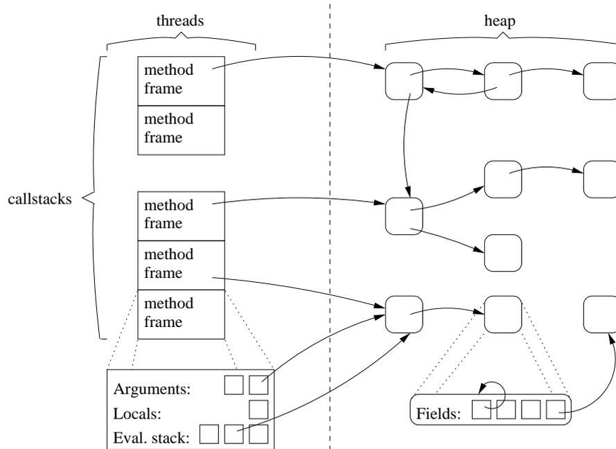
**Fig. 4.** Organisation of a state in a software model checker. It consists of two threads, each having a callstack. The three objects on the left are root objects, as they are referenced directly from the call stacks.
