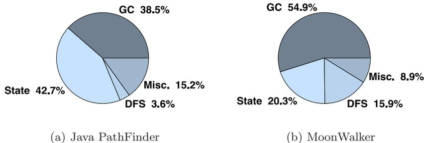
**Fig. 1.** Profiler data from Raytracer 3-1 benchmark [22] (see Section 4.2) describing the stakes of garbage collection (GC), state storage (State), exploration (DFS) and all remaining functionality (Misc.).
