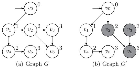
**Fig. 2.** Graph  $G$  was changed to graph  $G'$ , but the stored depths (the labels upper-right from the vertex) were not recomputed. Because of this, vertices  $v_2$ ,  $v_3$  and  $v_6$  are inconsistent, as indicated by the gray fill in graph  $G'$ .
