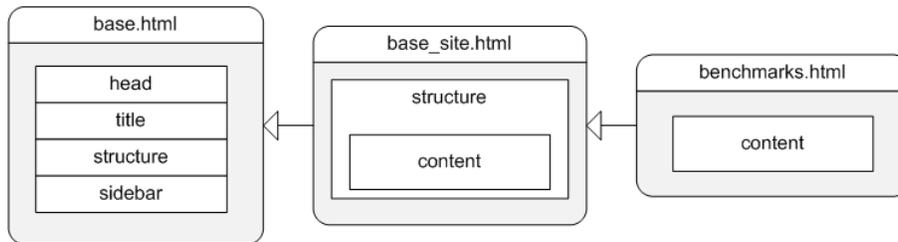
Figure 4.1: The basic template structure that is used for BeAT. Here `base_site.html` only extends the content block.
