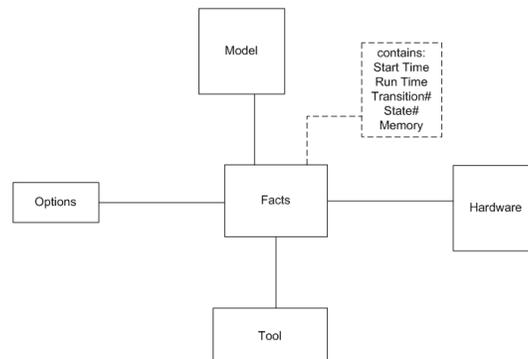
Figure 3.1: The initial, higher level database design, based on the data warehouse concept.
