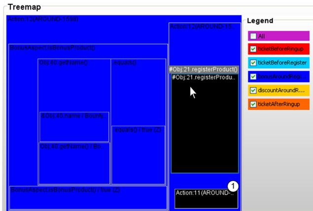
**Figure 5.9:** Trace visualization, showing the joinpoints that were skipped (in black) by the bonus aspect.
