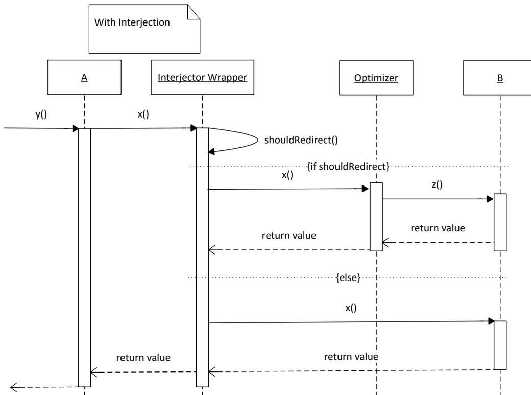
Figure 3.2.1.2 Interjector wrapper sequence diagram
