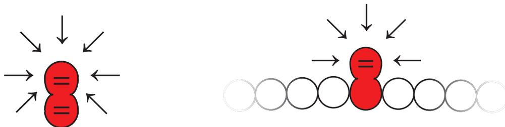
(a) Schematic representation of possible attack angles of a crosslinker that has not yet reacted.
