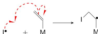
**Figure 2.13:** Electron rearrangement in radical addition reaction
