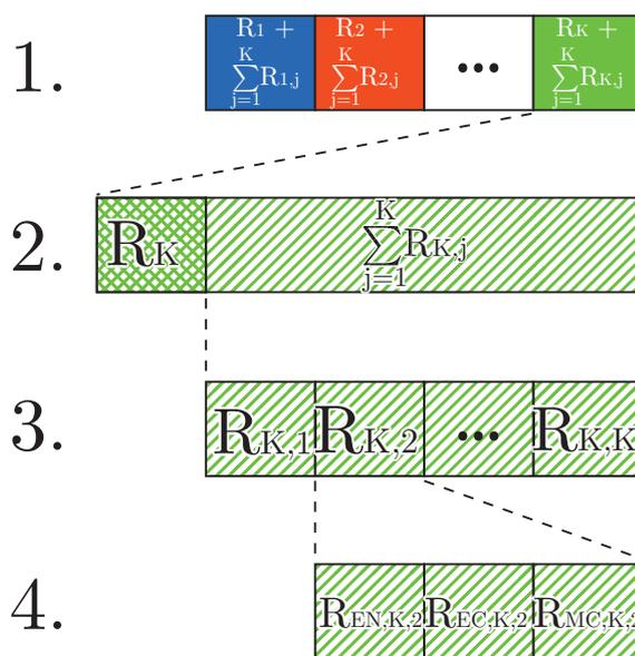
**Figure 5.2:** We perform multistage sampling by splitting up the sampling space, which is shown in Figure 5.1, by 1.) the radical species  $S_i$ , 2.) reaction type (intramolecular and intermolecular) 3.) vinyl species  $S_j$  (for intermolecular reactions) and 4.) the radical position  $Z \in \{EN, EC, MC\}$ . At each stage a sample is taken with the probability of each option depending on the reaction rates, yielding a reaction identified by  $Z, i$  and  $j$ .
