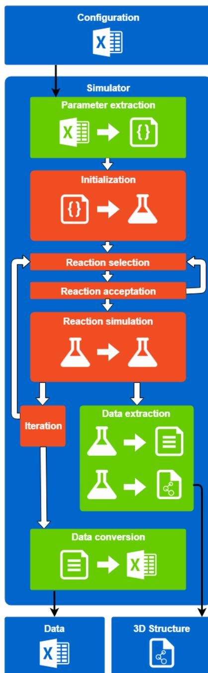
**Figure 6.1:** Program structure of our simulation. White arrows indicate program flow, black arrows indicate I/O. The separate files are indicated by the blue squares, internal I/O by green squares and the core algorithm in the orange squares.
