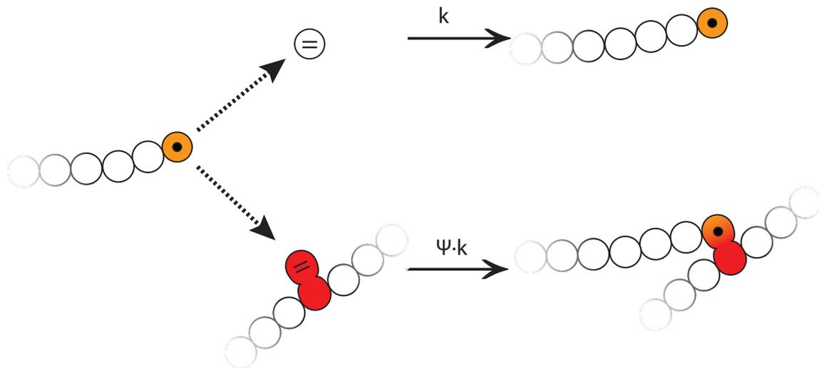
**Figure 4.2:** Schematic representation of propagation with a vinyl group in a crosslinker and a pendent vinyl group. The reaction rate of propagation with a pendent vinyl group has a factor  $\psi$  that is caused by the decreased accessibility of the vinyl group due to the polymer chain.
