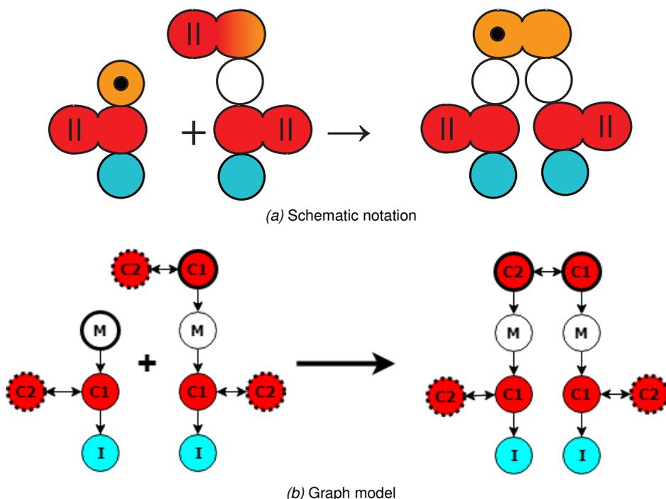
**Figure 5.8:** Example of crosslinking reaction in both the schematic notation of Chapter 1 and the equivalent graph models. The RAFT agent that is attached to the reactive center in the vinyl molecule is present, but not shown in the schematic notation.
