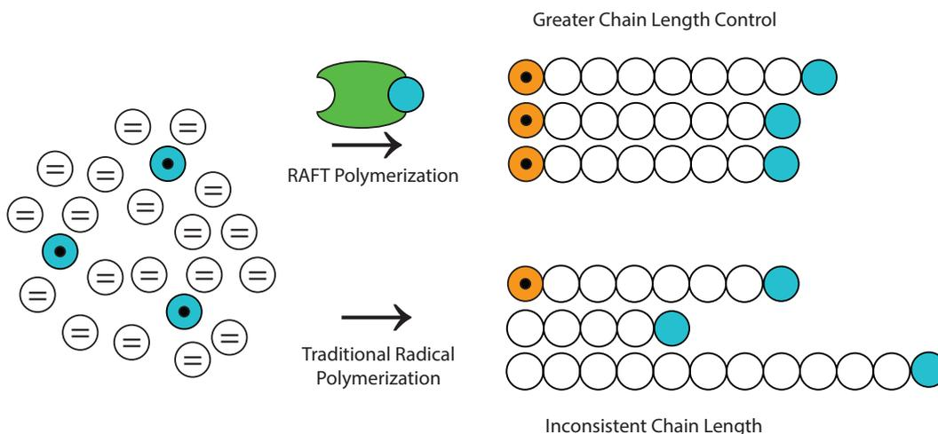
**Figure 1.9:** General comparison of polymers made with traditional radical polymerization against those made using RAFT process. Traditional radical polymerization also yields unreactive polymer chains due to termination. Recreated from [19].
