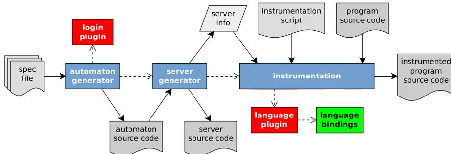
Figure 3.7: The full code generation process.
