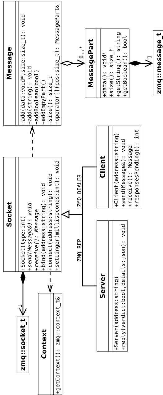
Figure 4.3: Class diagram for the inter-process communications library.
