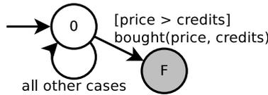
Figure 2.2: An automaton for example property 2. State ‘0’ is the initial state and the shaded state ‘F’ is the failure state. The image shows the values sent with the event and a conditional guard.
