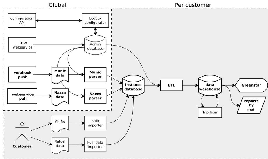
Figure 5.1: The data flows in the Shepherd platform.
