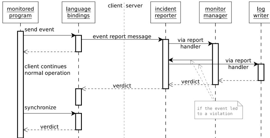
Figure 3.5: An example client-server interaction where the client tries to synchronize with the server, after the server has completed processing the message sent by the client. It shows that the logging call resulting from the failure as an asynchronous action, is completed before the synchronization point. What exactly happens with the message from the server is determined by the ZMTP implementation, but the message is retrieved in the synchronization function.
