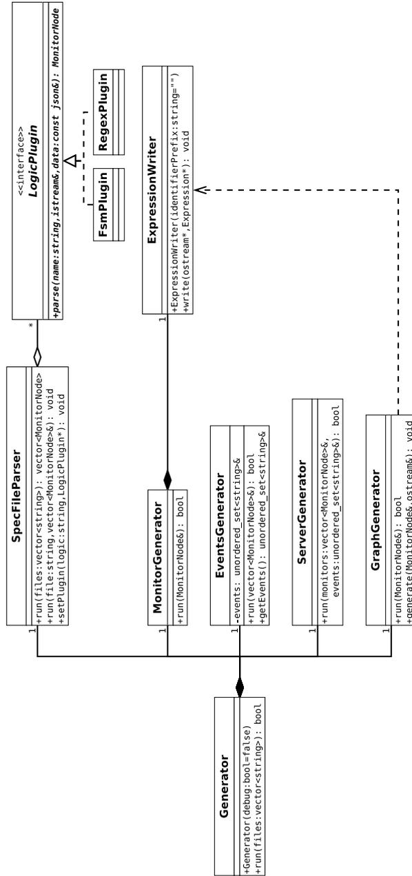
Figure 4.4: Class diagram for the code generation framework, plus two logic plugins.
