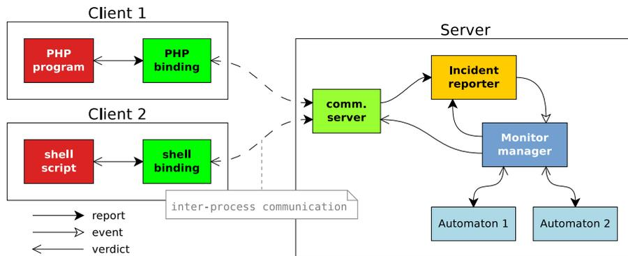
Figure 3.2: The full process resulting from a filed report, from the monitored program to the internals of the Sheepdog+ server.
