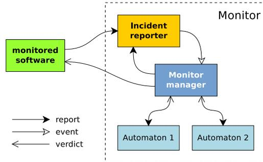
Figure 3.1: The interactions in the system as a result of the monitored software filing a report.
