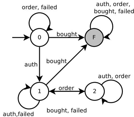
Figure 2.1: An automaton representing property 4 of the DSA example (“only after authentication and following a request can an order be successfully completed”). State ‘0’ is the initial state and the shaded state ‘F’ is the failure state.
