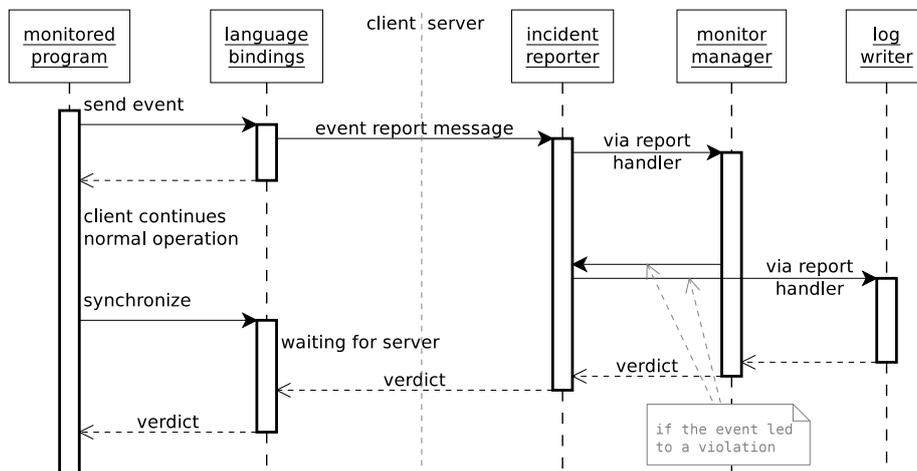
Figure 3.6: An example client-server interaction where the client tries to synchronize with the server, while the server is still processing the event. In this case the logging call is also completed before the synchronization point, because the server response only happens after all actions triggered by the event have completed.
