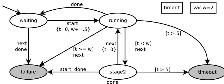
Figure 3.4: An example of a Sheepdog+ automaton. Guards are written between brackets and assignments are written between braces.  $\tau$  is not written explicitly on the transitions, but every transition without an event label is a  $\tau$ -transition. The shaded states are violation states.
