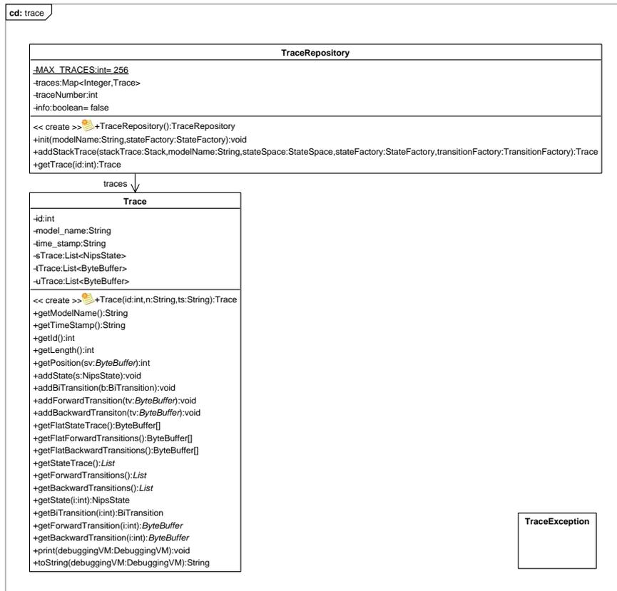
Figure 5.6: NIPS VM Trace Class Diagram
