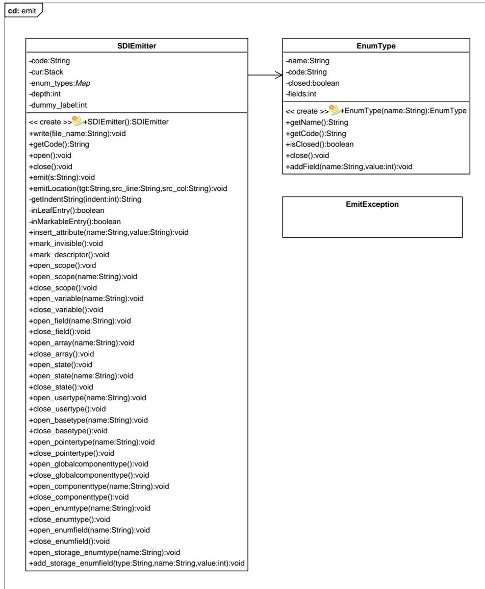
Figure 4.23: SDI Framework - *emit* package Class Diagram
