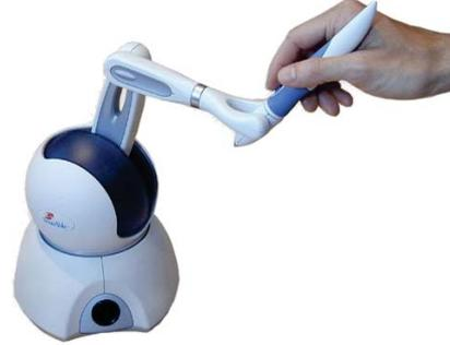
Figure 6. *SensAble<sup>®</sup> PHANTOM Omni<sup>®</sup>* haptic device with sensors in six degrees of freedom and actuators in three degrees of freedom, used for haptic user interaction.
